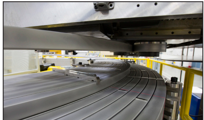
Superconducting magnet module in fabrication for ITER. Photo: GA
