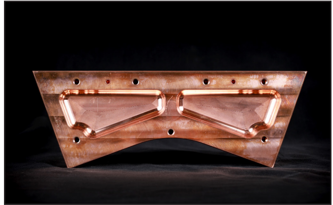
Component for high-powered microwave plasma heating system. Photo: US ITER/ORNL
