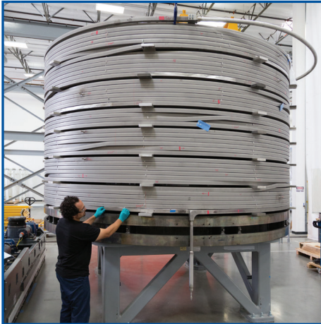
A module in the stack and join workstation. Photo: General Atomics
