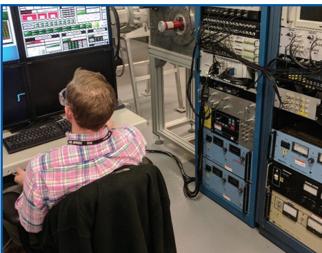
Control console and power supplies for Helmholtz coil arrangement. Photo: US ITER/ORNL
