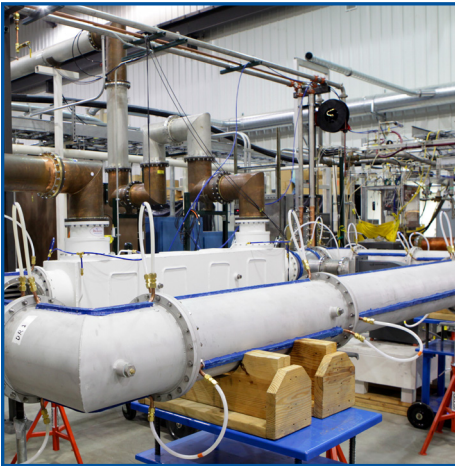
The resonant ring test stand at ORNL is used to test prototype components. Photo: US ITER
