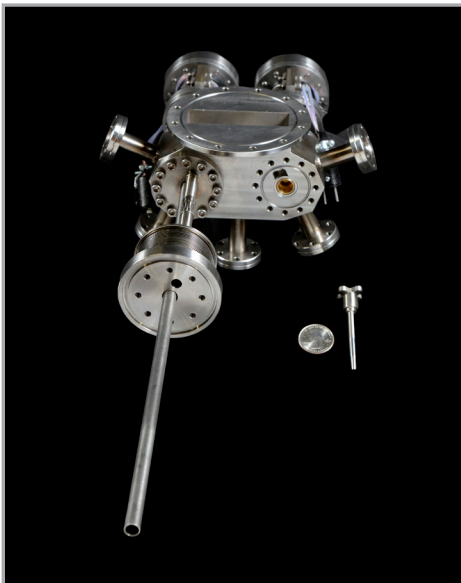
A dual-nozzle prototype was developed for fueling and ELM mitigation. Photo: US ITER/ORNL
