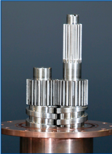
Close-up view of the twin-screw extruder. Photo: US ITER/ORNL
