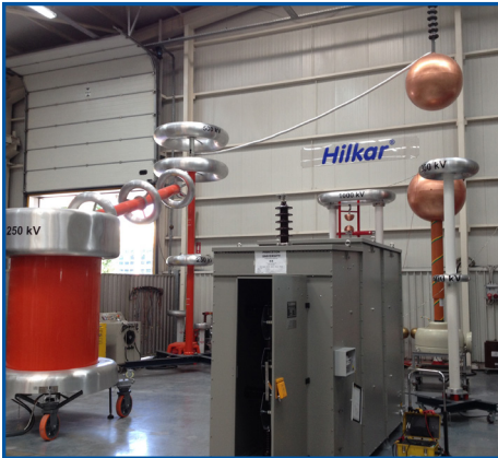
Earthing resistors during factory acceptance testing. Photo: US ITER
