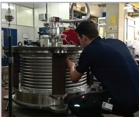
Factory acceptance testing of bellows. Photo: ITER Organization
