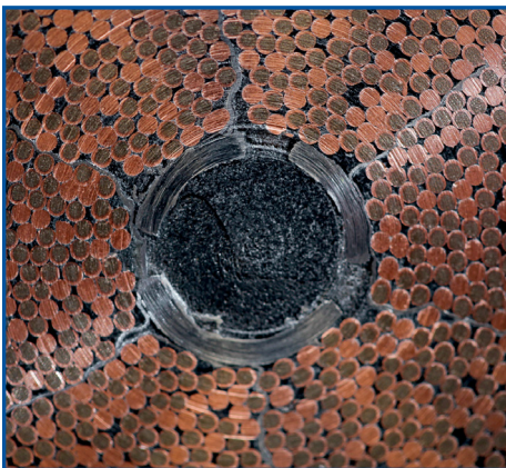
A close-up view of conductor shows the density of compacted strand around a helium cooling channel. Photo: US ITER
