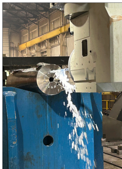
Precision long-bore drilling in a component of the low side field side reflectometer. Photo: General Atomics/Grand Valley Manufacturing
