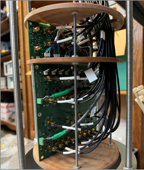
Neutron testing of operational amplifiers and level translators at Ohio State University Research Reactor. Photo: US ITER/OSURR
