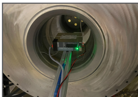
Static magnetic field testing of variable power supply. Photo: US ITER
