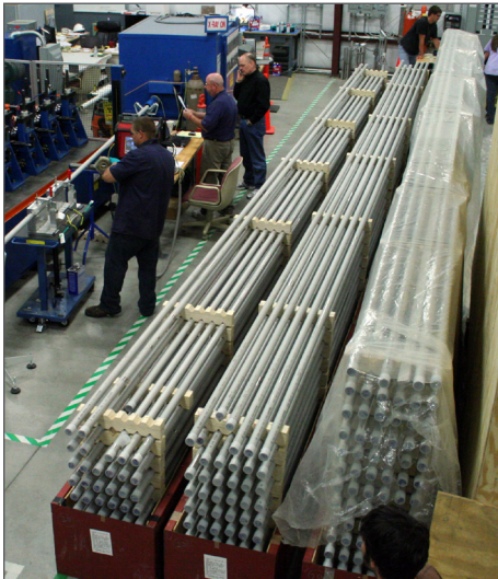
Jacketing material at the conductor integrator at the High Performance Magnetics facility. Photo: US ITER
