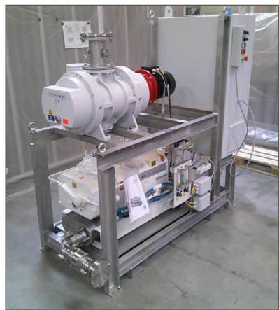
One of the non-active pump skids delivered to the ITER site in 2025. Photo: ITER
