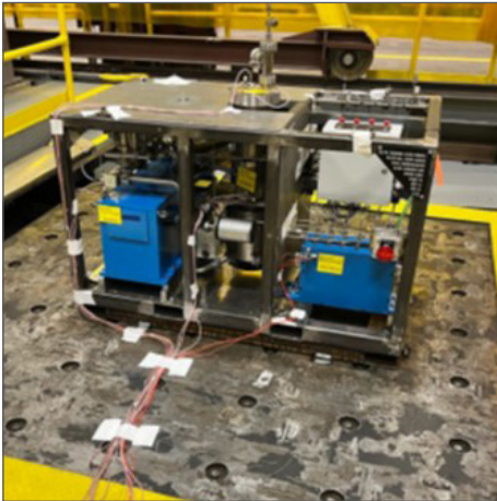
Seismic qualification of pump station for the cryogenic guard vacuum system. Photo: US ITER
