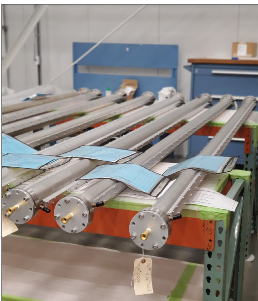
Sections of a waveguide. Photo: Teledyne Brown Engineering
