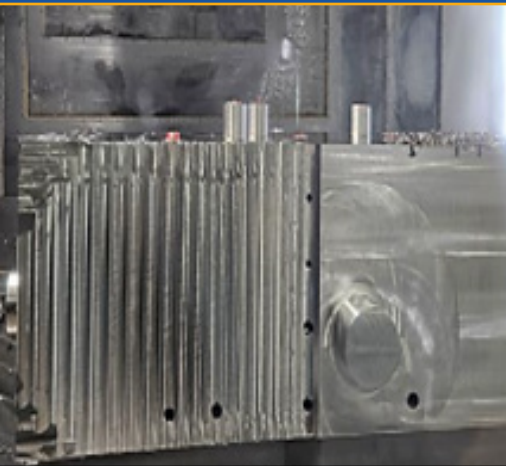
Gun-drilled block at start of pre-weld machining of antenna block for the low field side reflectometer. Photo: US ITER/Keller Technology
