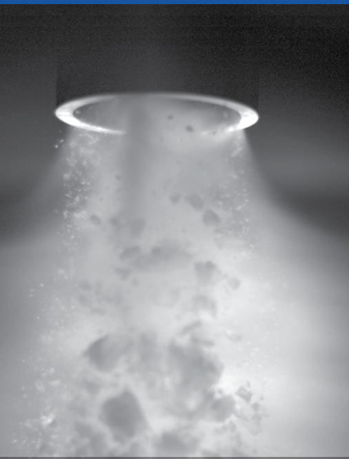
Pellet fragments exiting the shatter tube of the test bed. Photo: ORNL
