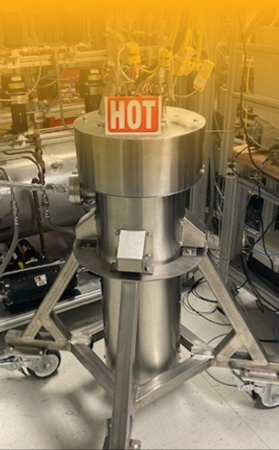
Testing of an ambient molecular sieve bed. Photo: US ITER
